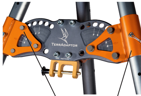
Fig 7 Offset Leg Clamps (left-facing forward; right-facing backwards) for illustrative purposes. Best practices has both offset leg clamps facing forward in a typical tripod configuration set up
