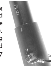
Fig 3 Improperly Secured Leg Coupling Pin
